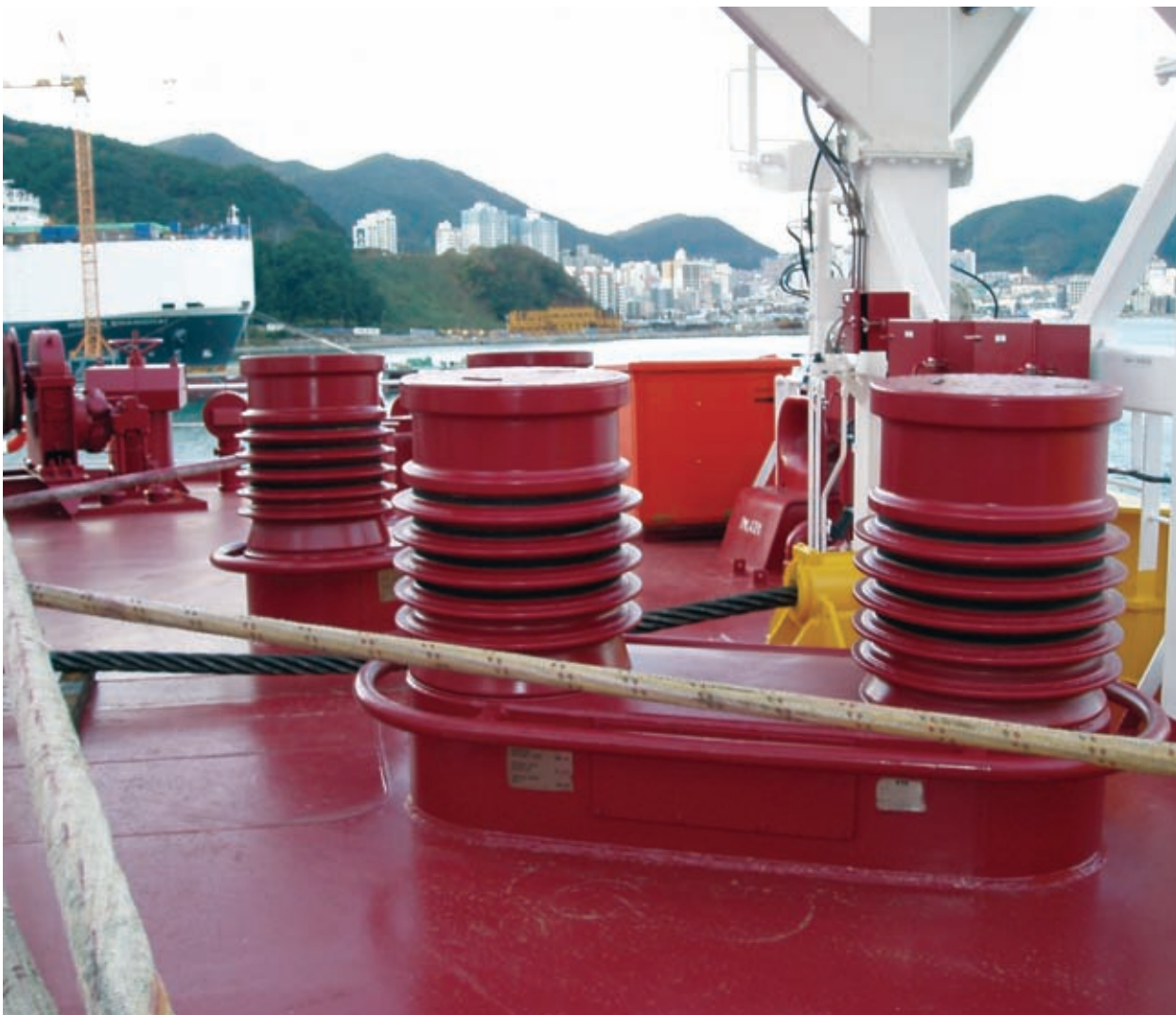
The stern section of one of the Vela VLCCs showing TTS' Winch Bollards in place.
