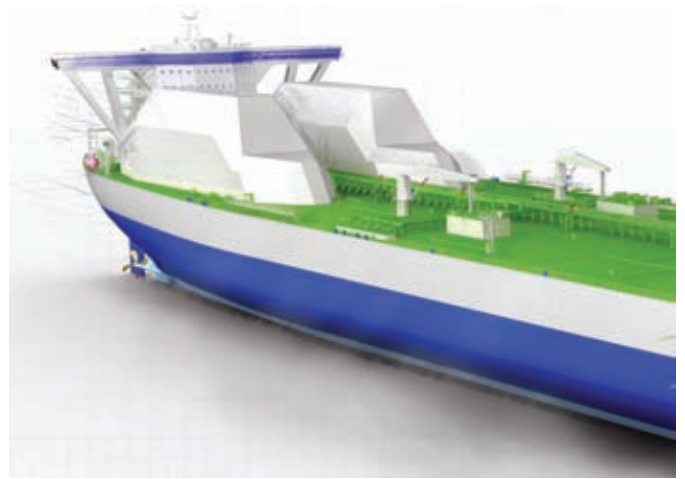
Two gas tanks are fitted on the deck ahead of the accommodation block.
